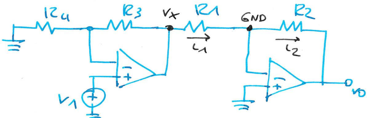
$$I_1 = \frac{v_x}{R_1} = -\frac{v_0}{R_2} = I_2 \quad ; \quad v_0 = -\frac{R_2}{R_1} v_x = -\frac{R_2}{R_1} \left(1 + \frac{R_3}{R_4}\right) v_1$$
