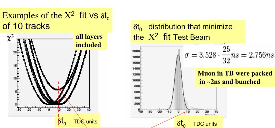
$\delta t_0$  of min  $X^2$  fit for one track
