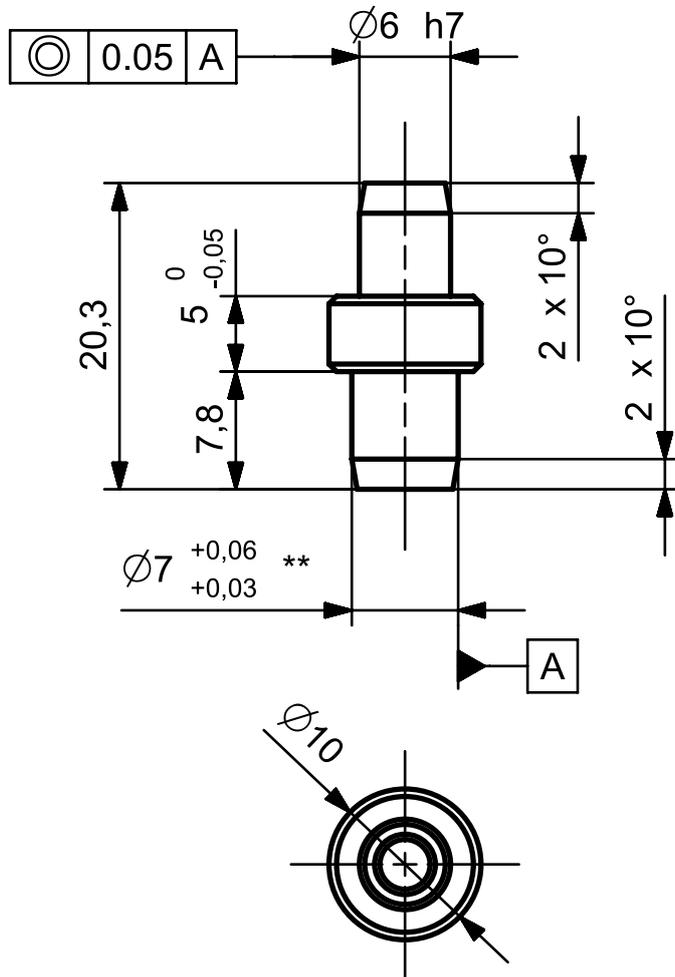
**\*\* N.B. IL CILINDRO  $\varnothing 7 \times 7,8$  DEVE ESSERE ACCOPPIATO CON INTERFERENZA NELLA SEDE  $\varnothing 7$  DELLE PIASTRE GUIDA**
