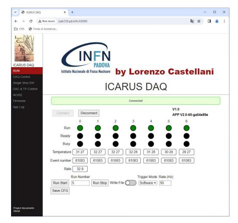
2) From the DAQ Control page and the DAC & TP Control page you can change the contents of the various registers of the A2795 cards detected in the MINICRATE.
