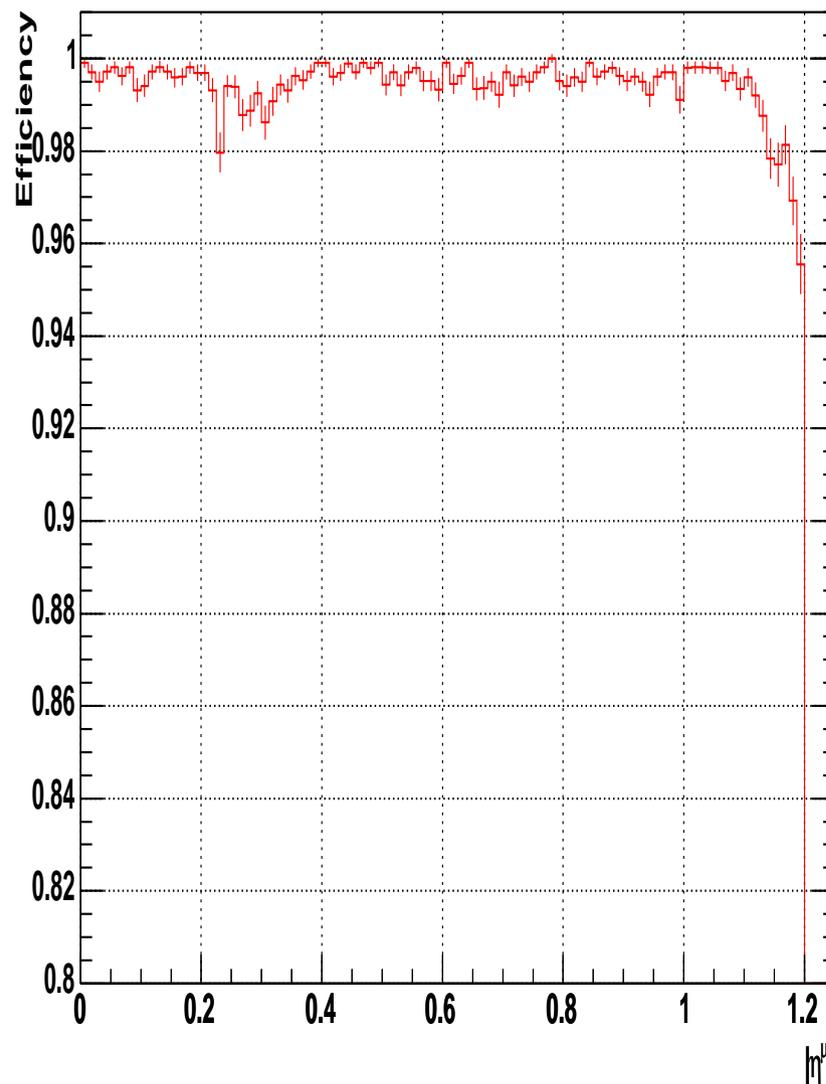
Single Muon,  $p_t = 5 \div 100 \text{ GeV}/c^2$ ,  $|\eta| < 1.2$  **Eff GMR/SA**
