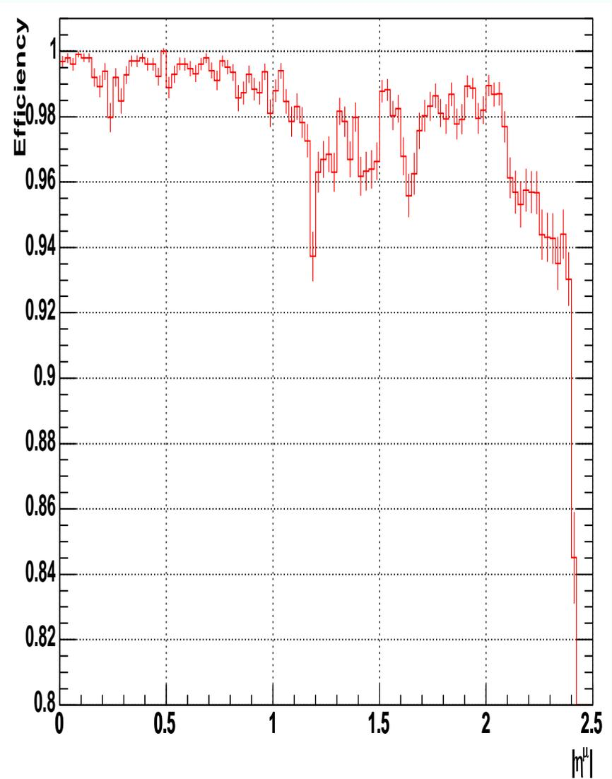
Single Muon,  $p_T = 1 \text{ TeV}/c^2$ ,  $|\eta| < 2.4$  **Eff GMR/SA**
