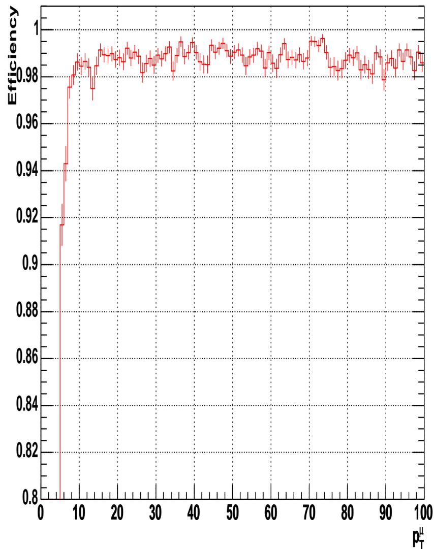
Single Muon,  $p_t = 5 \div 100 \text{ GeV}/c^2$ ,  $|\eta| < 1.2$  **Eff L3/L2**
