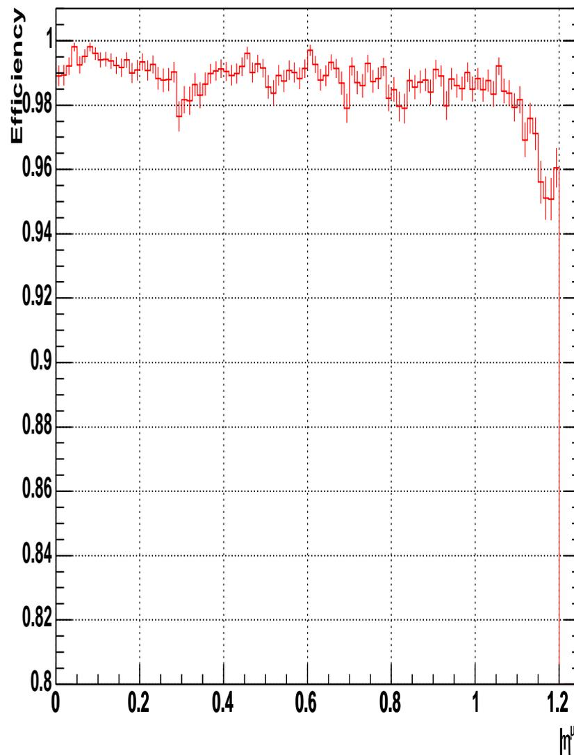
Single Muon,  $5 \div 100 \text{ GeV}/c^2$ ,  $|\eta| < 1.2$  **Eff L3/L2**
