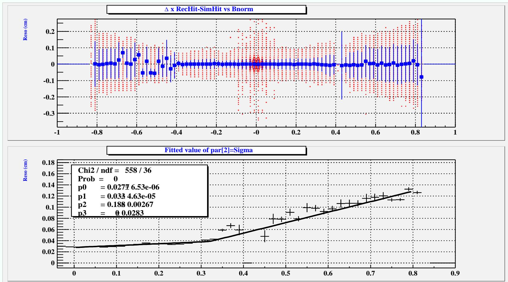
Resolution for  $\theta \approx 0$ ,  $B_{\perp} \approx 0$  is  $\sigma \approx 280 \mu m$ .
