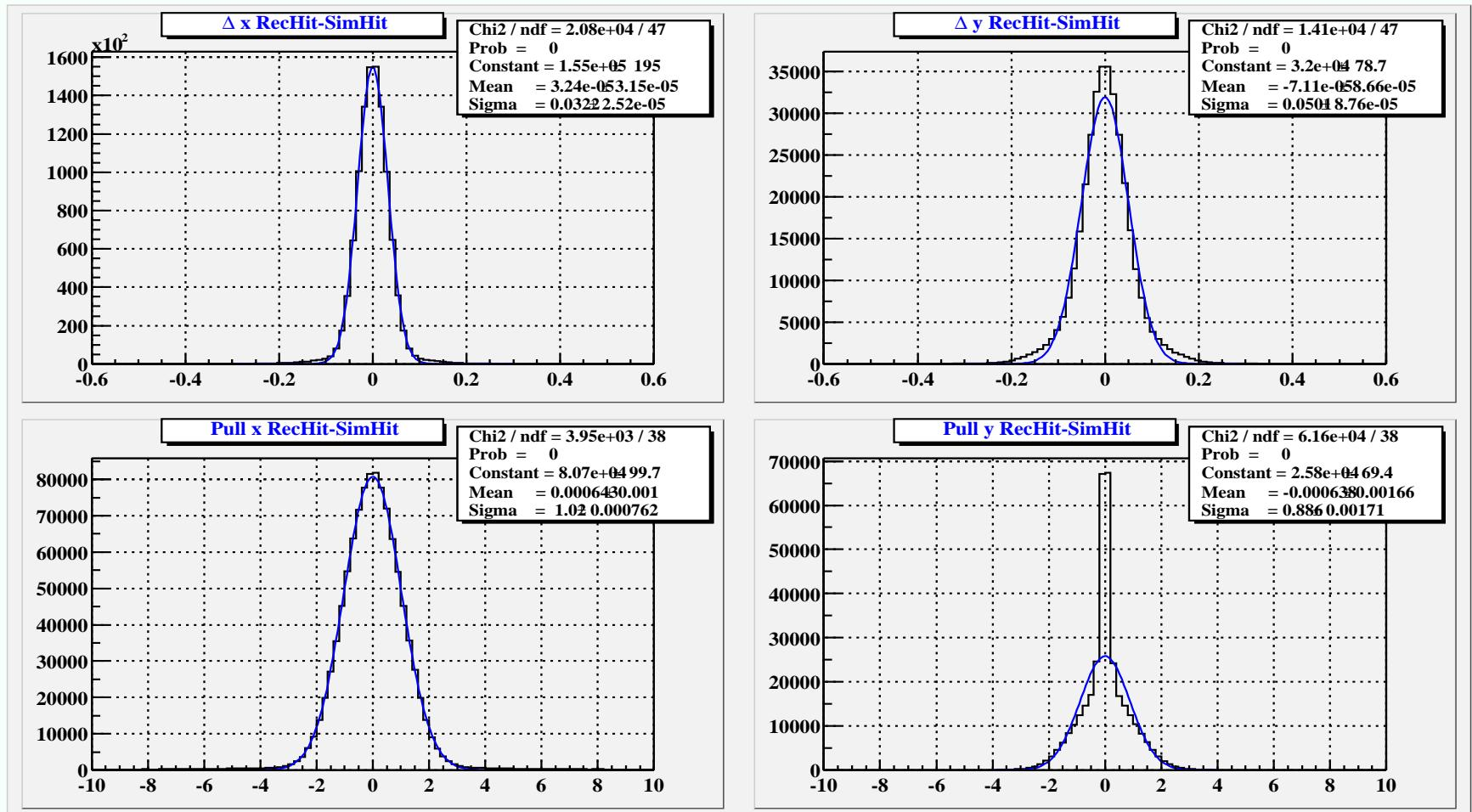
$$\sigma(Pull) \approx 1.02 \text{ for } \phi \text{ SL}, \sigma(Pull) \approx 0.88 \text{ for ZED SL}$$
