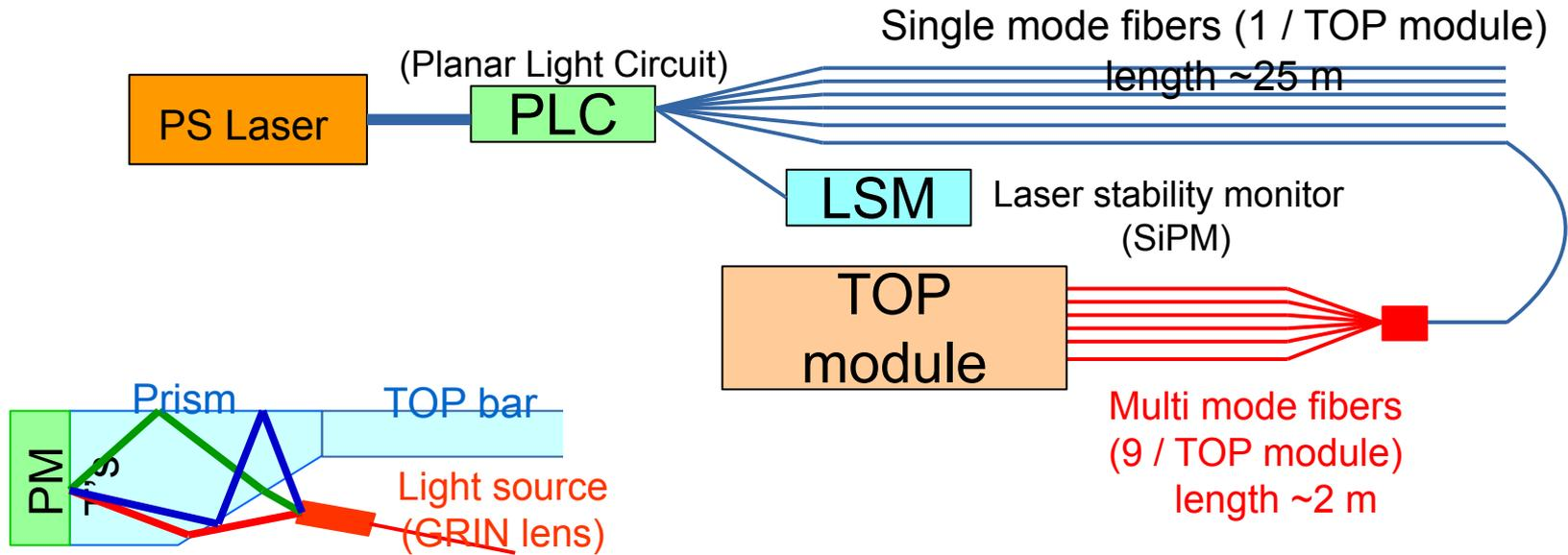
A PMT pixel can be reached by different light paths (with different times)
