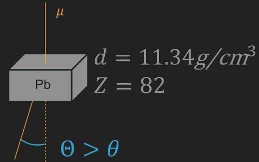
Muons are highly penetrant, using multiple scattering we can build 3D maps of inaccessible, large volumes
