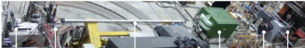
target Be or C   Si microstrip stations   vacuum beam pipe   dipole magnet   CAL   DT
