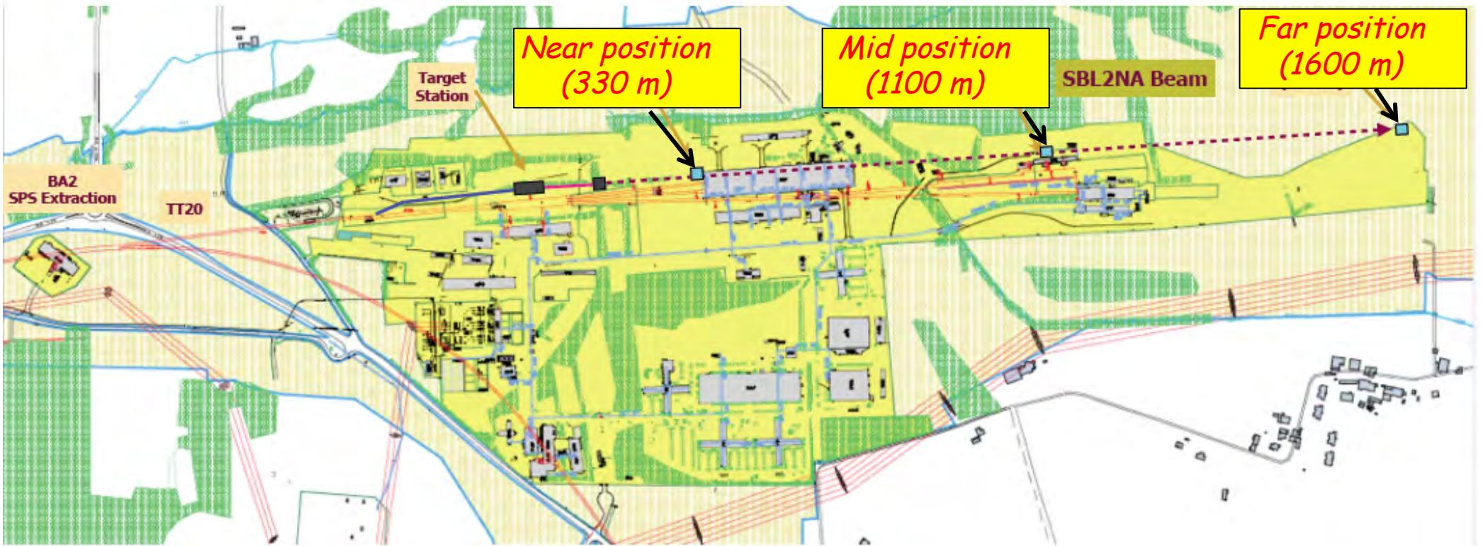
100 GeV primary beam fast extracted from SPS; target station next to TCC2; decay pipe  $l = 100\text{m}$ ,  $\varnothing = 3\text{m}$ ; beam dump: 15m of Fe with graphite core, followed by  $\mu$  stations.
