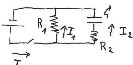
$$a) I(0) = V_0 \frac{R_1 + R_2}{R_1 \cdot R_2}$$
