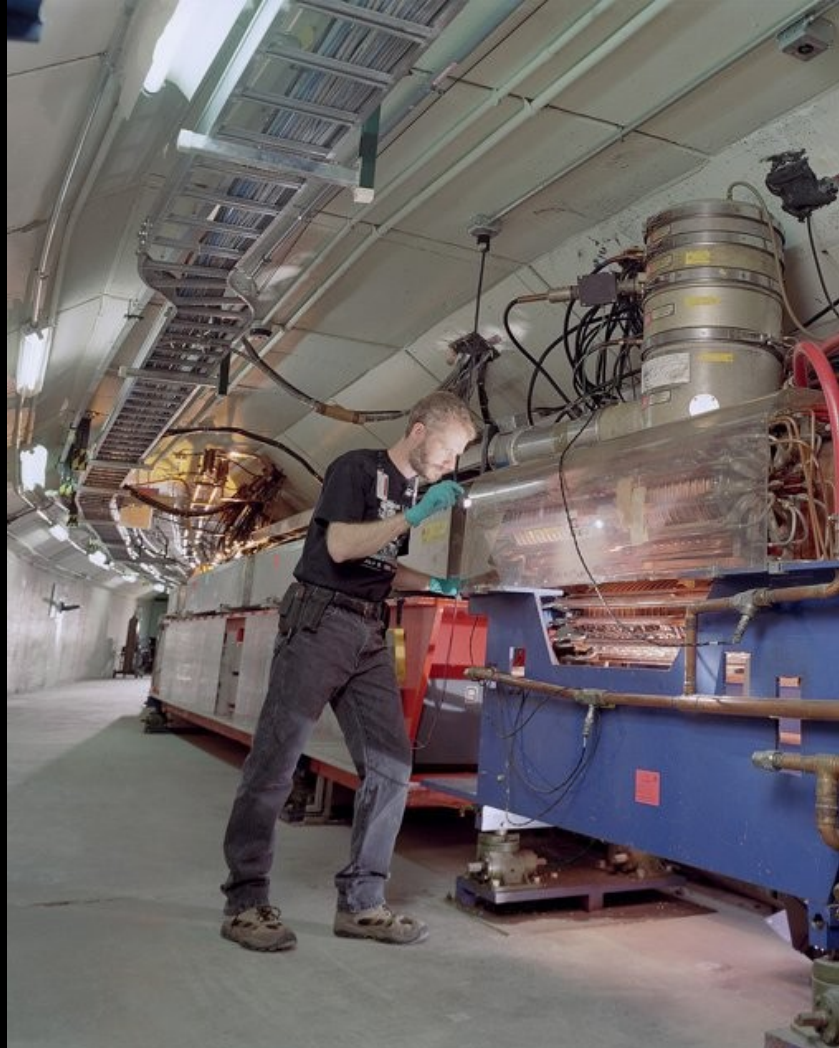
The Booster synchrotron strips electrons off H^- and accelerates remaining protons up to 8 GeV
