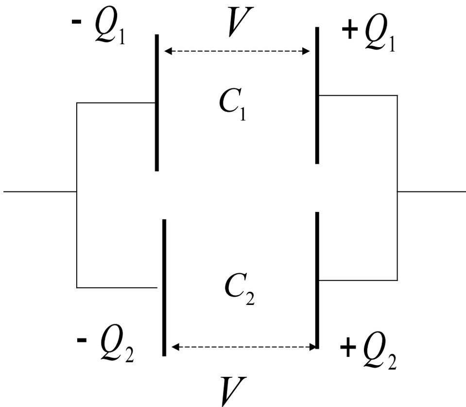
$$Q_1 = C_1 V \quad Q_2 = C_2 V$$
