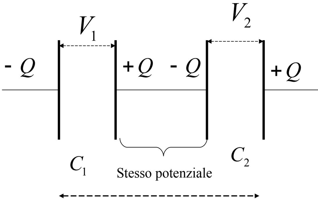
$$V = V_1 + V_2$$
