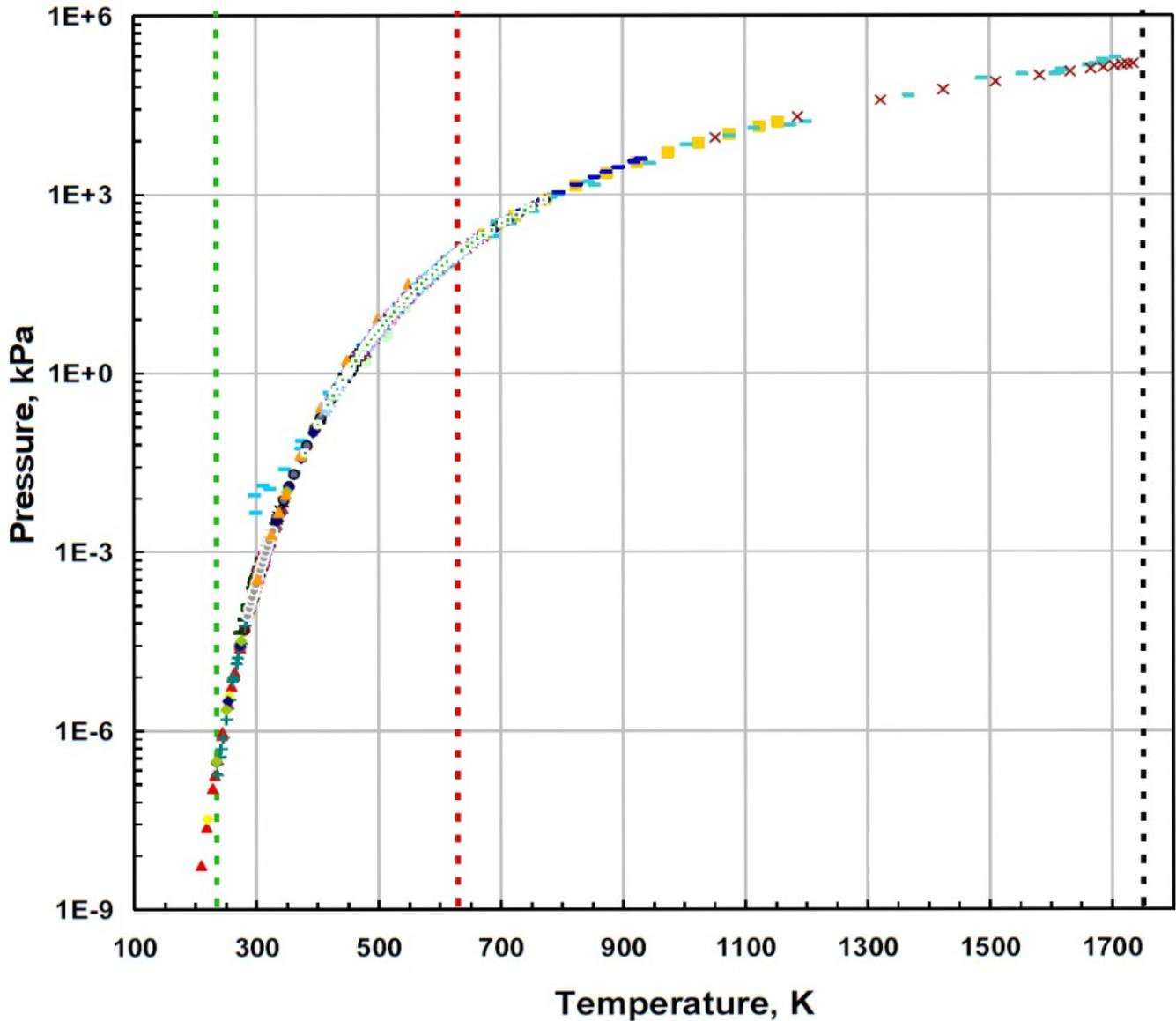
Figure 1. Experimental vapor pressure data for mercury.
