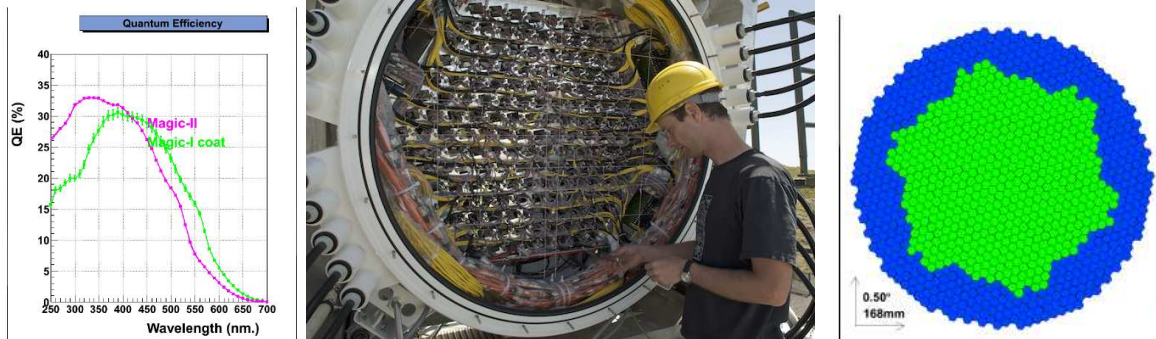
Figure 2.5: The MAGIC II camera, trigger and photomultipliers photocathode efficiency.
