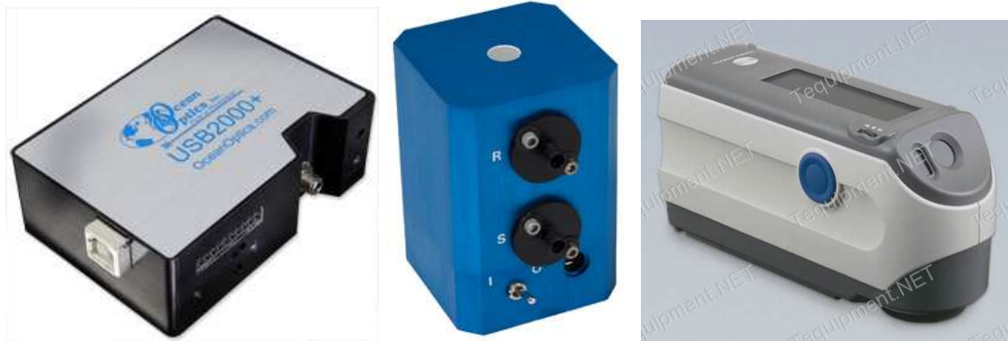
Figure 4.18: (left) Ocean Optics USB2000+ Miniature Fiber Optic Spectrometer and ISP-REF Integrating Sphere, (right) Minolta spectrophotometer CM-2600d.
