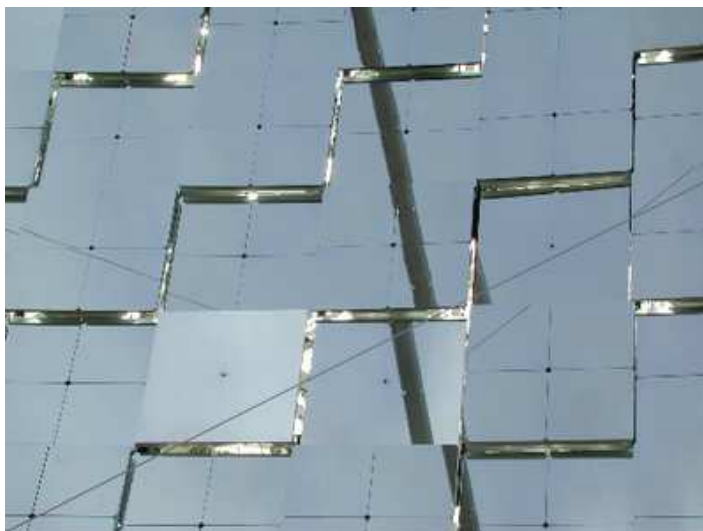
Figure 3.13: The staggering of MAGIC I mirrors. The mirrors are shifted 60 mm forward or 20 mm backward with respect to the original position, without causing any degradation in image reconstruction.
