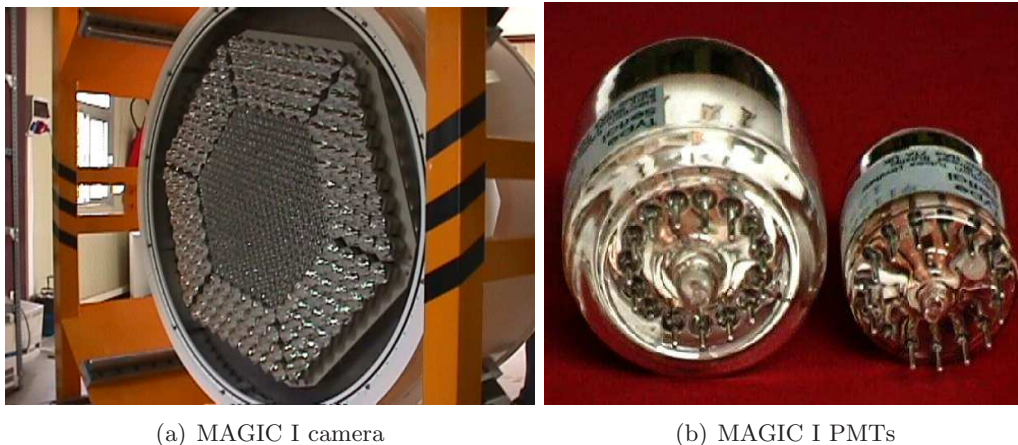
Figure 2.4: The camera system of MAGIC I. In figure (a), the camera before shipment. Inner and outer pixels, shown in figure (b), are mounted. The light-catchers (Winston-cones) are also mounted in front of the pixels. In figure (b), the two types of Electron Tubes PMT are shown. The larger one (1.5' \varnothing ) is mounted on the outermost part of the camera, the smaller pixels (1' \varnothing ) are mounted in the central part.
