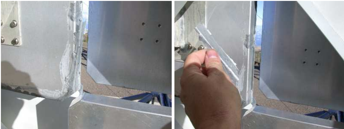
Figure 4.32: Detachment of the UV-paint on prototypes MAGIC II aluminum mirrors mounted on MAGIC I.
