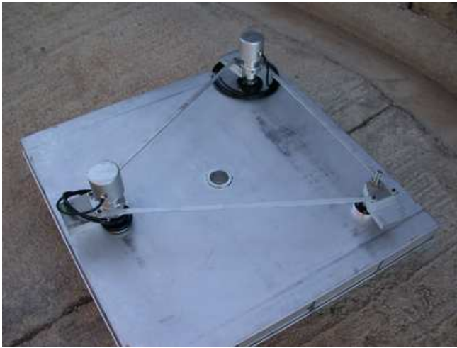
Figure 4.33: The AMC actuators mounted on the back of the aluminum mirror before mirror installation. There are three types of fixations, all with ball bearings: one fixed point (bottom-right), one single-cardanic point (top-right) and one bi-cardanic point (left). The hole at the laser will host the AMC laser.
