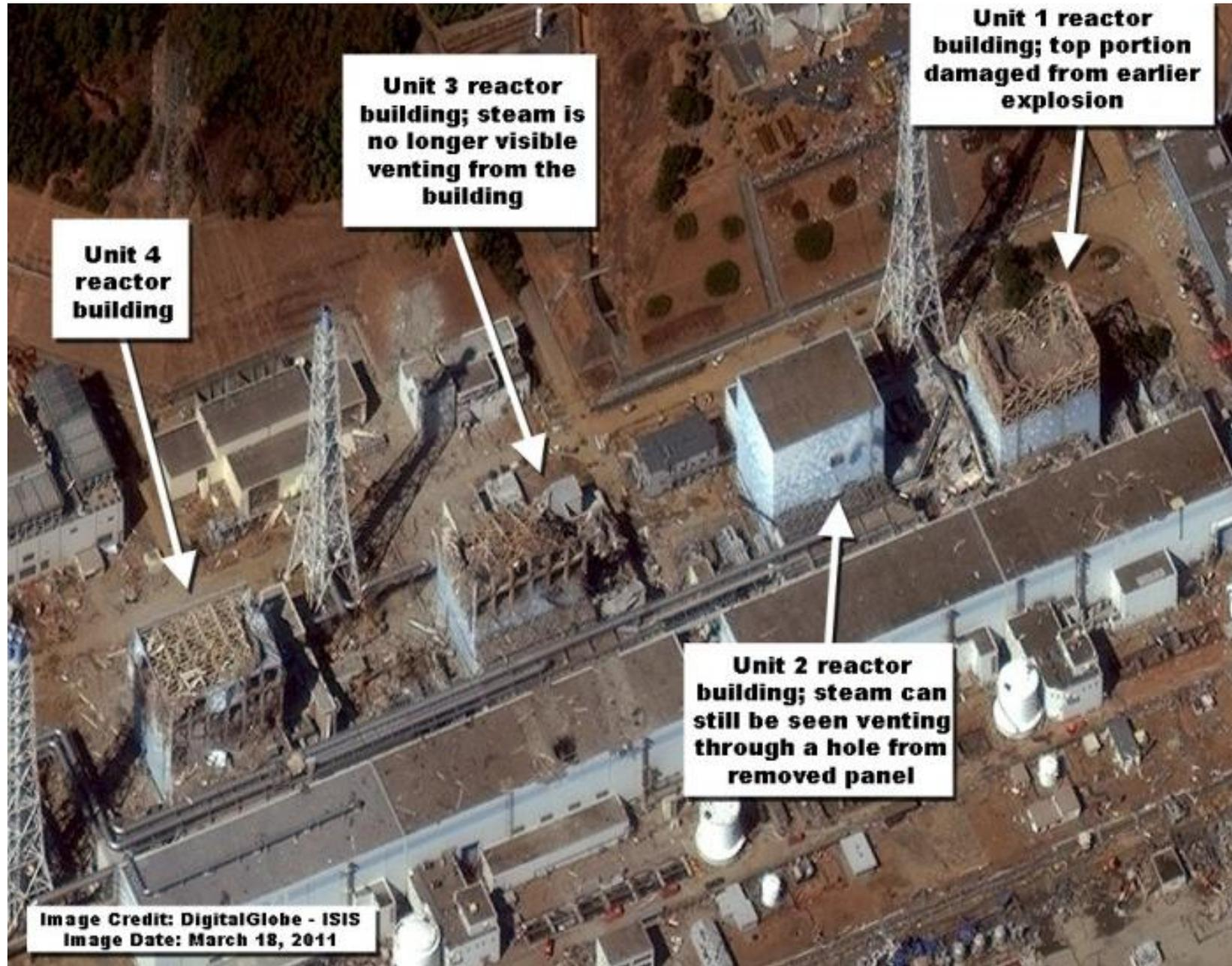
**Unit 1 reactor building; top portion damaged from earlier explosion**
