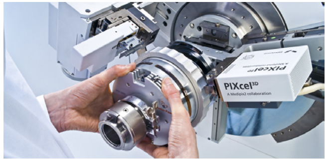
Figure 41. PANalytical PIXcel detector system, based on single-chip Medipix2 technology, developed in collaboration with Nikhef. The Empyrean X-ray diffractometer in which these detectors are used, received an R&D award of R&D Magazine in 2011.
