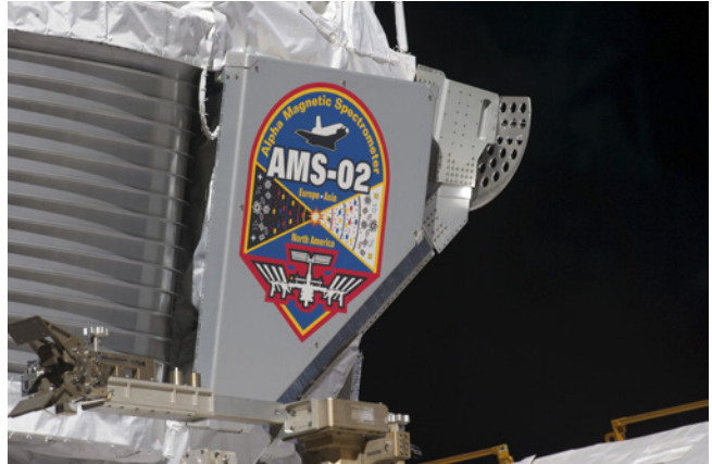
Figure 40. The AMS-02 detector mounted on the International Space Station ISS. The CO 2 -cooling system for the silicon trackers of this experiment was developed by Nikhef in collaboration with NLR.
