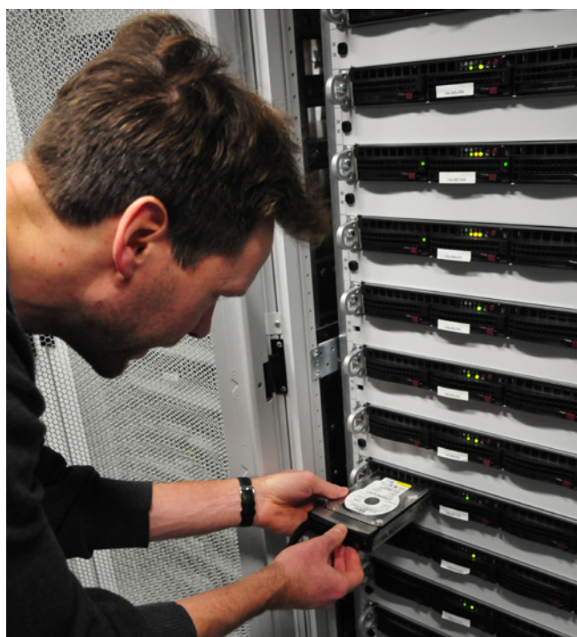
Figure 39. A member of the Grid Computing Group replaces a harddisk in one of the Tier-1 storage modules.
