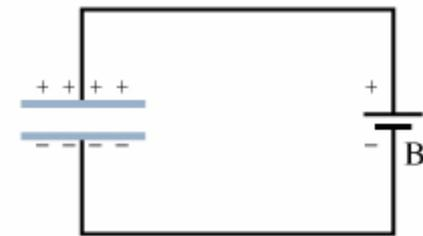
$$U_1 = \frac{1}{2} \frac{q_1^2}{C_1} = \frac{1}{2} C_1 V^2$$
