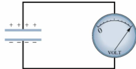
$$U_1 = \frac{1}{2} \frac{q^2}{C_1} = \frac{1}{2} C_1 V_1^2$$
