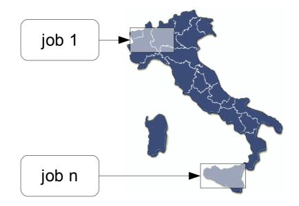
A fundamental piece for the Grid-ified RISICO system is the gJobSubmitter module, which takes care of setting up all needed thing for jobs to run, basing on preferences specified in a configuration file. This module, when launched, uploads files into the Storage Elements, creates a jdl file for each job and submits the jobs itself. Then it follows their execution until it terminates, retrieving produced output for each succesfully terminated job.
